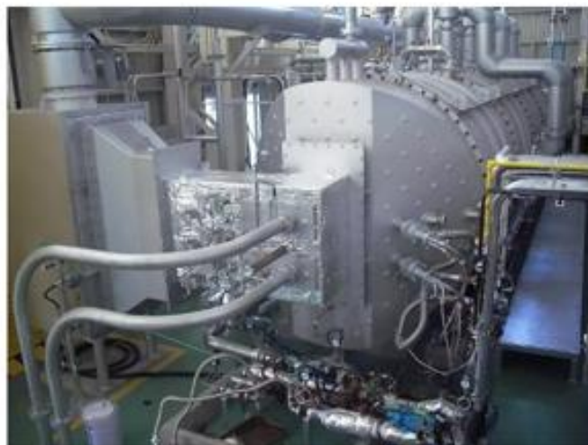
Ammonia combustion test equipment (0.5t/h furnace)
